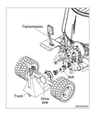
④ Remove drive axle mounting bolts from the frame and then slowly pull out the truck with drive axle to the front.
