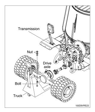
⑤ Remove drive shaft from the transmission by loosening the mounting bolts.
